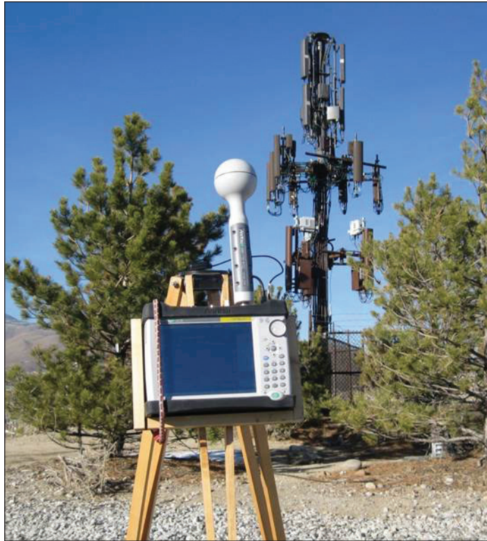
Figure 10. Receiver BER performance in the field is affected by ambient RF noise
